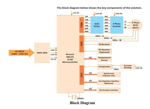
Solutions include the hardware and controller firmware for BLDC motor and IR receiver. The switch mode power supply (SMPS) is capable of operating from 190V - 270V AC.
